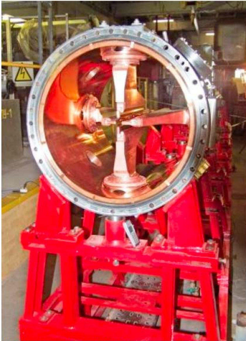
Figure 2: view of the RFQ with open outlet flange
