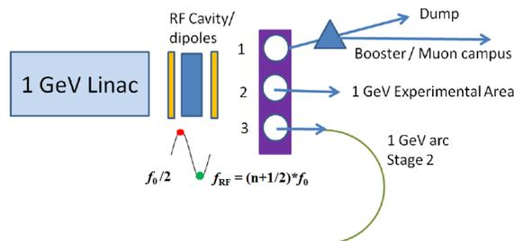
Figure 4: Conceptual design of 1 GeV extraction line.
