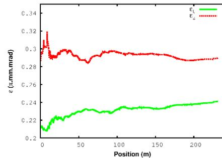
Figure 7: Longitudinal (green) and transverse (purple) beam emittance through stage 1.
