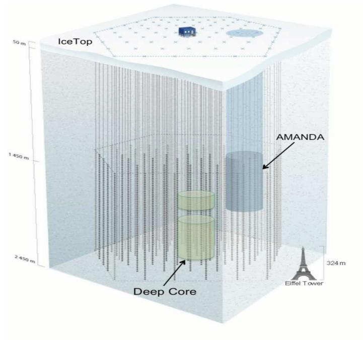
ICECUBE, 1 Km3 of insrumented ice by 2011, 80 strings of Digital Optical Modules, 59 of which have been installed.  ICECUBE, 1 Km3 of insrumented ice by 2011, 80 strings of Digital Optical Modules, 59 of which have been installed.
