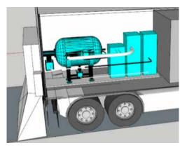
Fermilab's technology will deliver a high-throughput, portable, scalable and cost-effective solution to treatment of a wide variety of chemical contaminants and pathogens. The compact electron-beam accelerator being developed at Fermilab can be deployed on a portable skid for in situ treatment.
